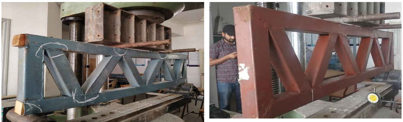
Figure No 3: Failure of Cold Form Steel and Hot Rolled Steel
