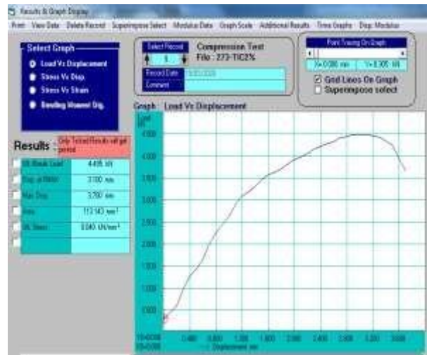
Figure 5. Compression strength of Mg with 2% TiC matrix
