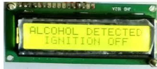
Fig. 8. LCD Display of Alcohol Detection
