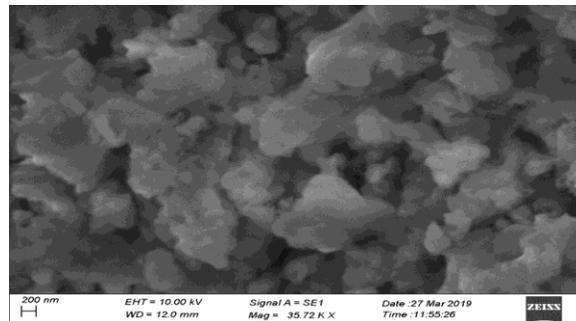
Fig. 5. SEM images of biosynthesized CuNPs of *C. guianensis* (a). Flower Petals (b). Stem (c) Bark and (d) Leaves.
