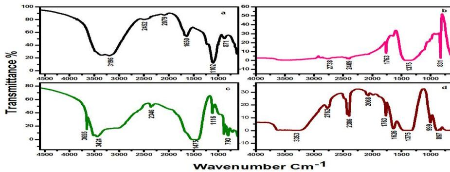
Fig.4. FTIR spectrums of CuNPs made from couroupita guianensis (a). Flower Petals (b). Stem (c) Bark and (d) Leaves
