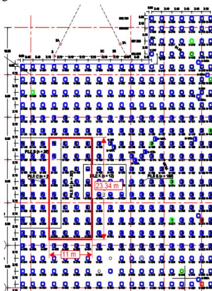
Fig. 5 Pile layout of tabletop foundation Turbine-1
