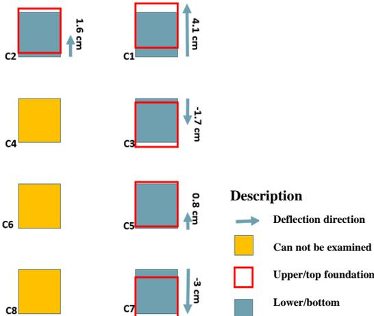
Fig. 8 Verticality check on foundation slope and tilting
