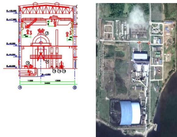
Fig. 3 Geometry and layout of tabletop foundation Turbine-1
