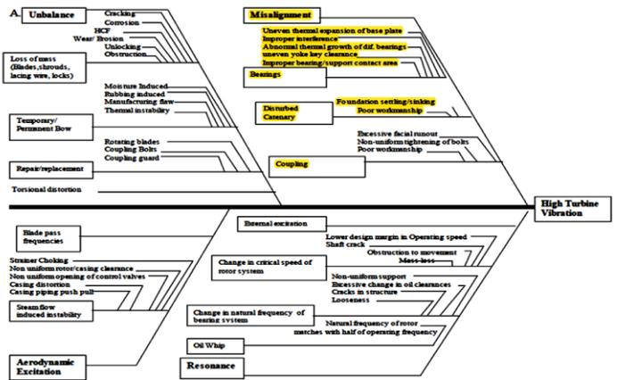
Fig. 10 Fish bone diagram of turbine vibration problems-I
