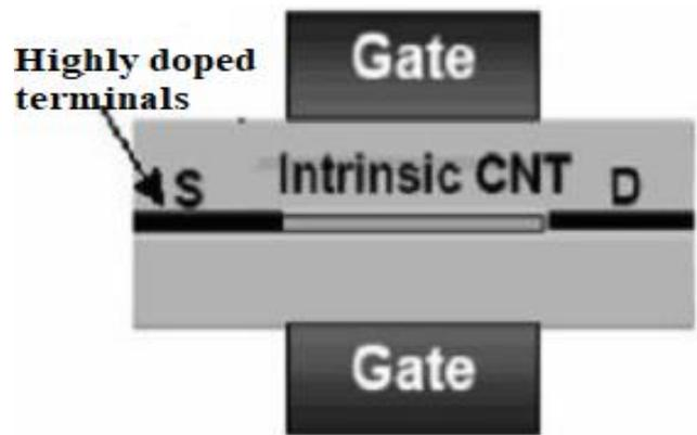
Figure 7: MOSFET like CNTFET structure [20]
