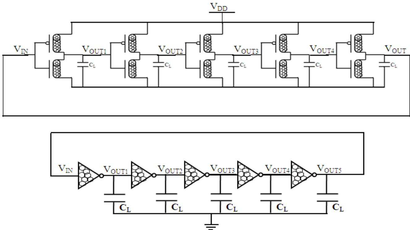
Figure 8. CNTFET based ring oscillator [25]
