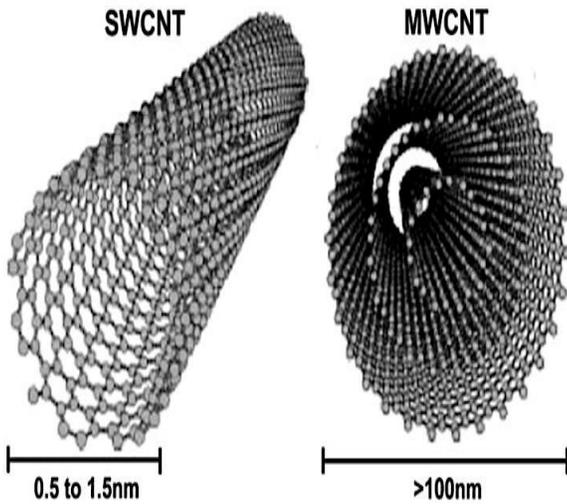
Figure 2. Single walled and Multi walled carbon nanotube [5]
