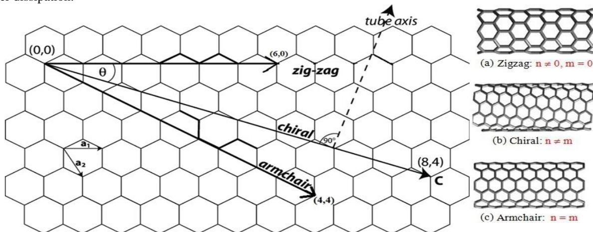
Figure 1. Geometry of carbon nanotube and its different configurations
