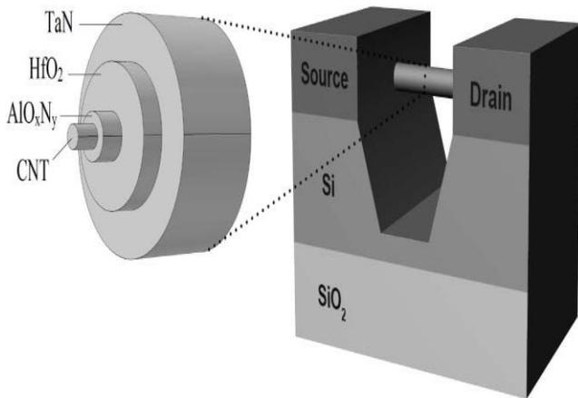
Figure 5.Wrap-gate CNTFET structure [13]
