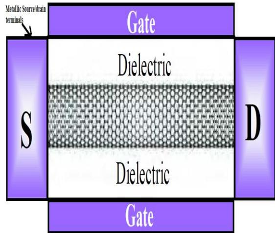
Figure 6: Schottky barrier CNTFET with metallic source/drain [16]
