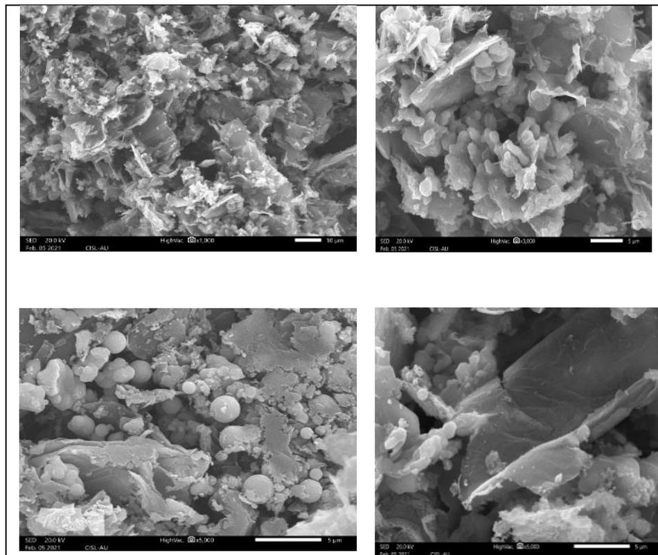
**Figure 3.4: SEM analysis of GO and GO Composites Mn<sub>3</sub>O<sub>4</sub> with a mass percent of 50:50**
