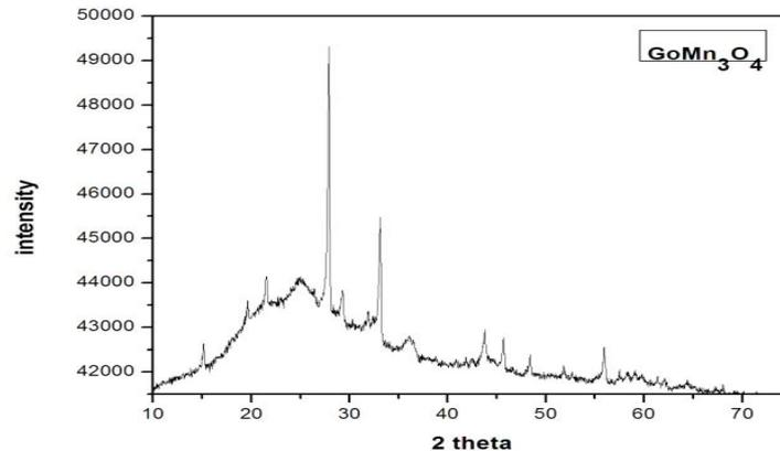
**The XRD pattern of  $\text{Mn}_3\text{O}_4$  nanoparticles is shown in Figure. 3.1b**
