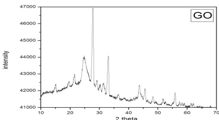
Figure 3.1 XRD pattern of Nano Graphene Oxide
