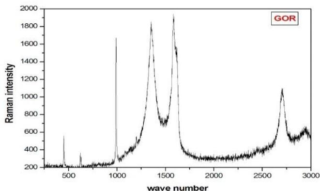
**Fig.3.3 Raman spectra Nano Graphene Oxide**
