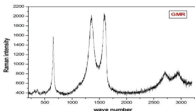
**Fig 3.3 b GO/Mn<sub>3</sub>O<sub>4</sub> composite Raman spectra of 50:50 ratio.**
