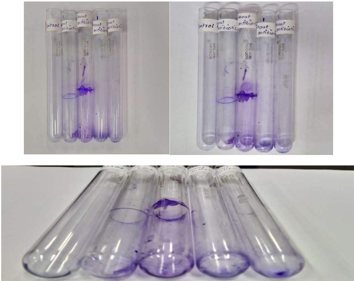
Figure 1: Tube method qualitative assay used for the detection of biofilm producing organisms because of occurrence of visible biofilm. The crystal violet used here stains the biofilm formed by the organism so that the results can be easily visualized.
