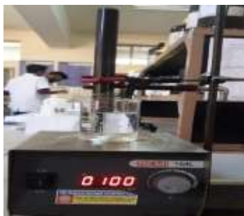
Figure 10: modified In-vitro drug release study assembly
