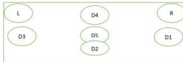
Figure 1. Schematic representation of measurements of optical densities at various spots on an X-ray film.
