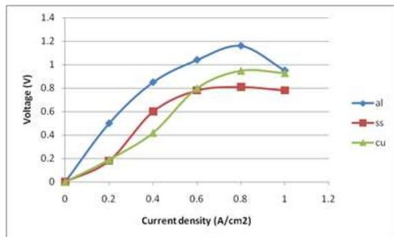
Figure 25: Polarization Curve for Three Bipolar Materials
