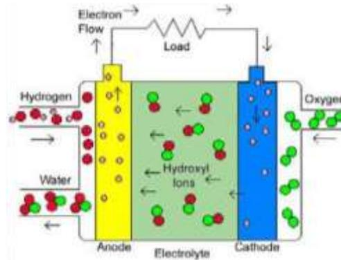
Figure 3: Schematic Diagram of AFC
