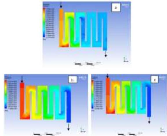
Figure 20: Pressure distribution at the anode region for each material with temperature 323 K at 2.5 bar: (a) Aluminum, (b) Copper, (c) Steel.
