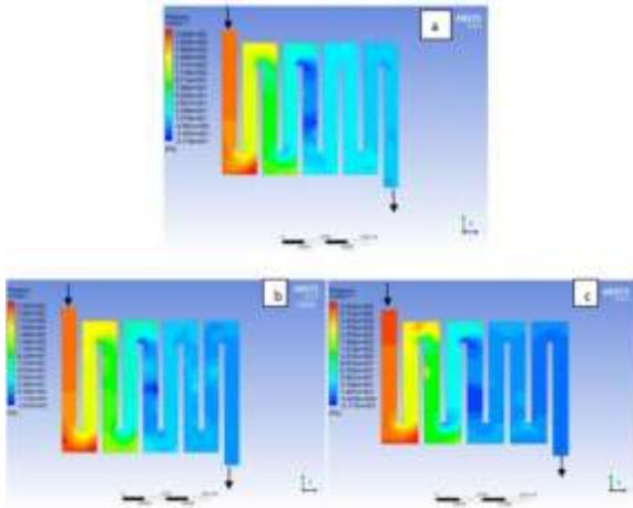
Figure 18: Pressure distribution at the anode region (GDL/CL) for each material with temperature 323 K at 2.0 bar: (a) Aluminum, (b) Copper, (c) Steel.
