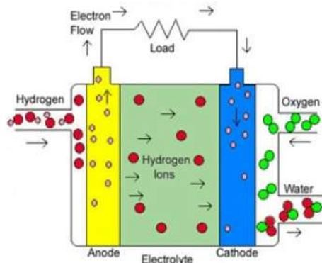
Figure 2: Schematic Diagram of PEMFC
