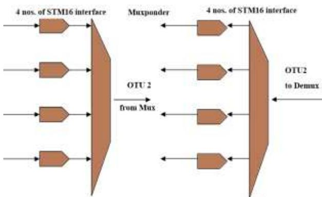
Fig. 4. TX & RX Muxponder interfaces details-type-I
