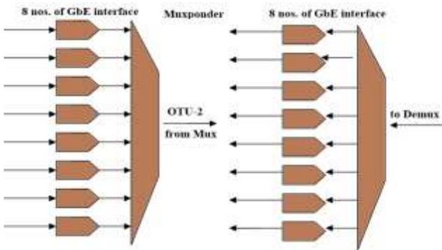
Fig. 5. TX & RX Muxponder interfaces details-type-II
