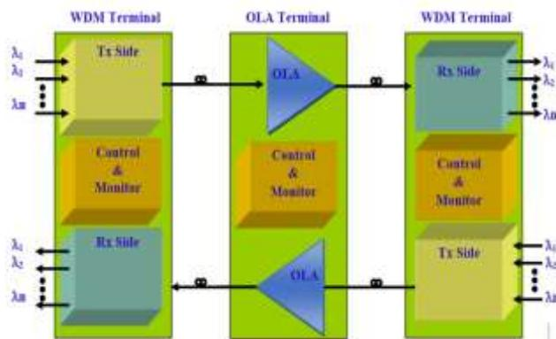
Fig. 1. DWDM system block diagram
