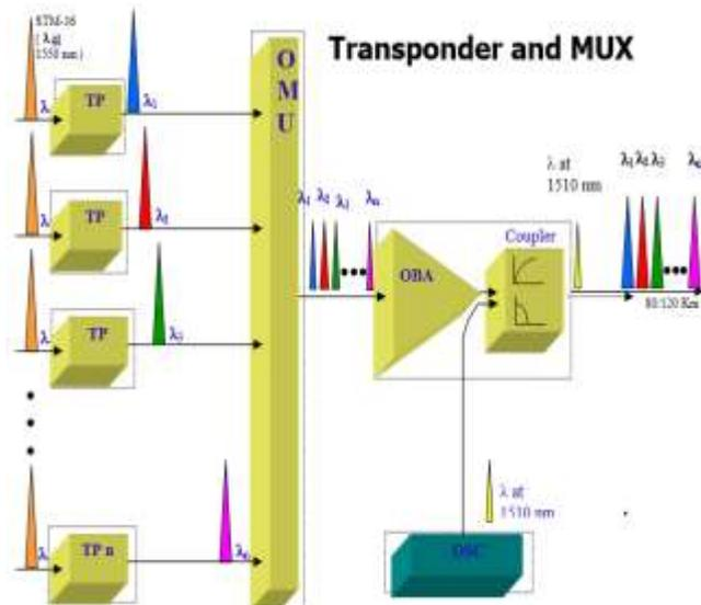
Fig. 2. Transponder block diagram with MUX
