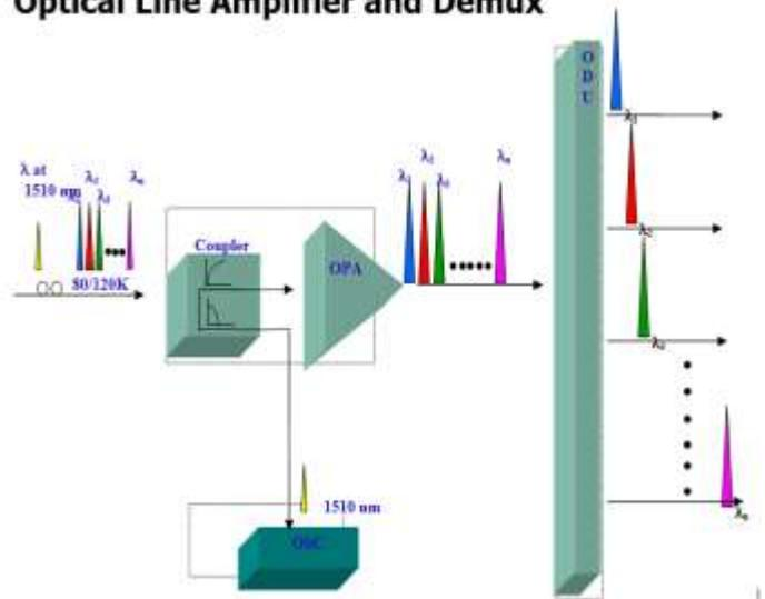
Fig. 3. Transponder block diagram with DeMUX
