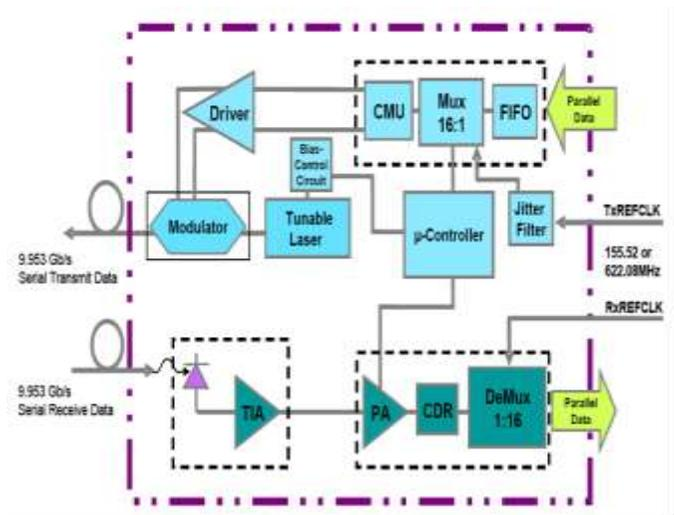
Fig.8. functional block diagram of transceiver [16]
