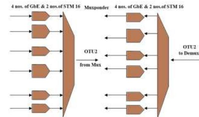
Fig.6. TX & RX Muxponder interfaces details-type-III
