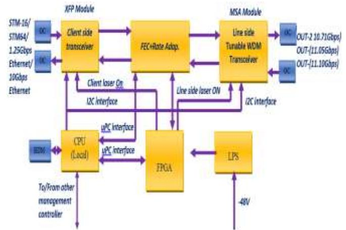
Fig.7. hardware schematic of transponder
