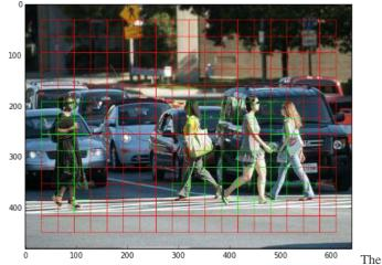
There are many grid cells of same dimensions withinside the picture above. When an object arrives within a grid cell, every grid cell will notice it. If an object centre occurs within a grid cell, the grid cell will become green, indicating that this cell is responsible for detecting it.
