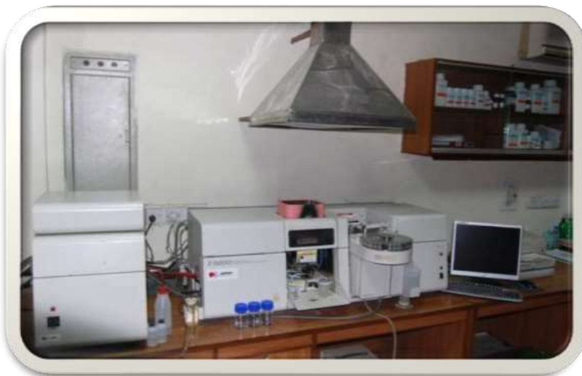
Figure 2: Hitachi Polarized Zeeman AAS, Z-8200, Japan
