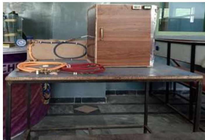
Figure 2: Actual experimental setup of LPG refrigerator
