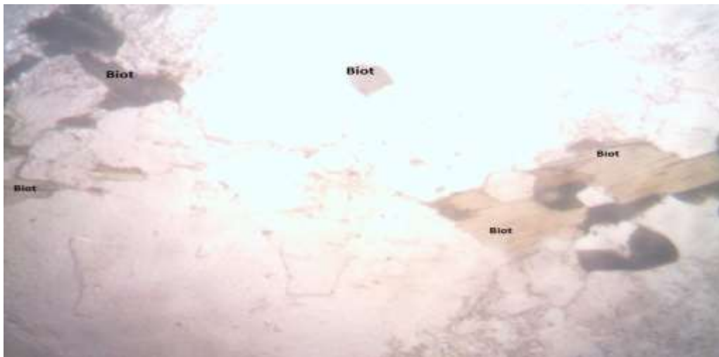
Plate 2: Photomicrograph of Biotite Granite in plane polarised light (Biot).
