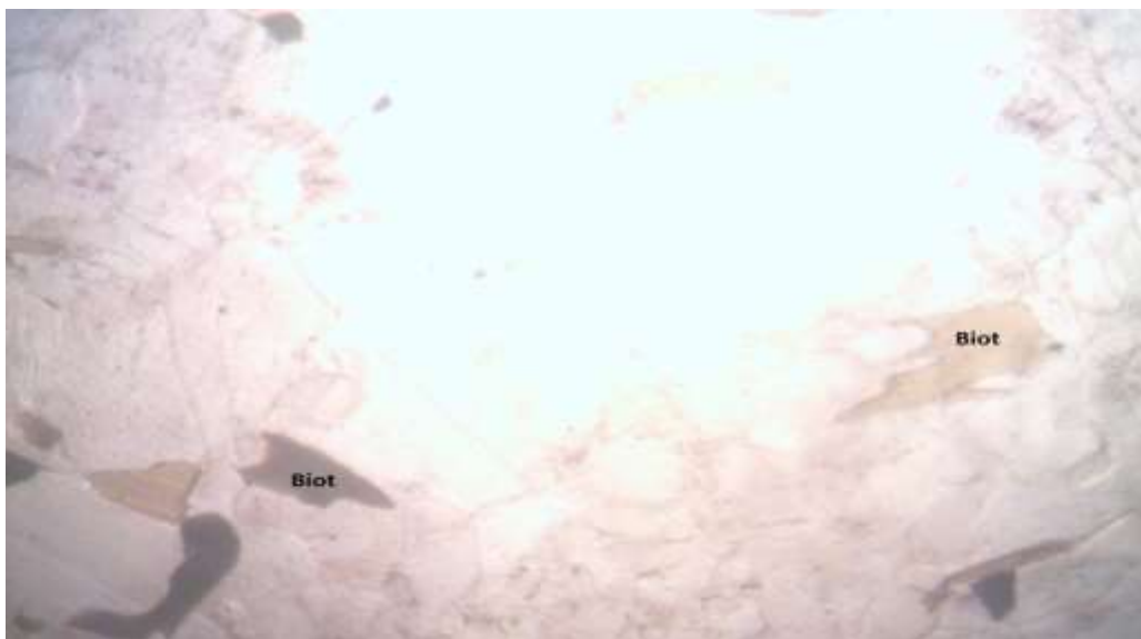
Plate 4: Photomicrograph of Biotite granite in plane polarised light showing Biotite (Biot).
