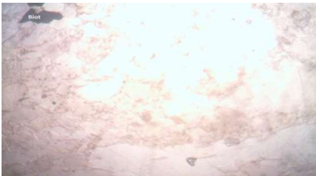
Plate 6: Photomicrograph of Granite in plane polarised light showing biotite (Biot).
