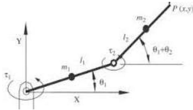
Figure 1 : Position and orientation of robot kinematic linkage
