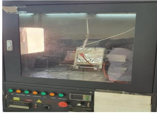
Figure 1: electrospinning /electrospray system (Nano NC, ESB200, South Korea)
