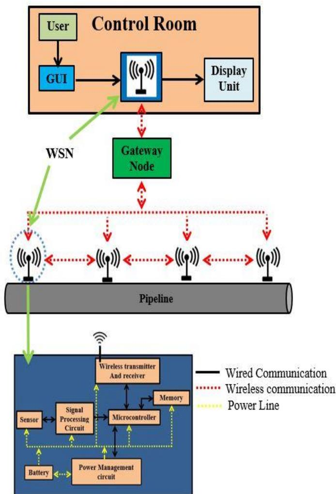
Figure. 1: IoT based Pipeline monitoring system
