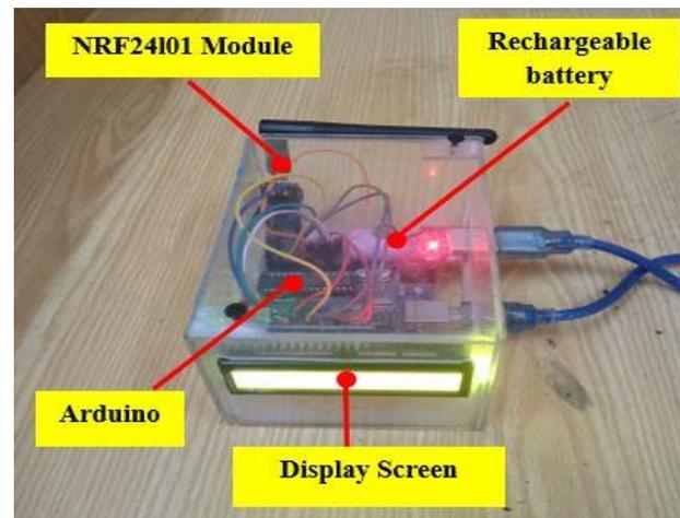
Figure. 4: Wireless receiver unit
