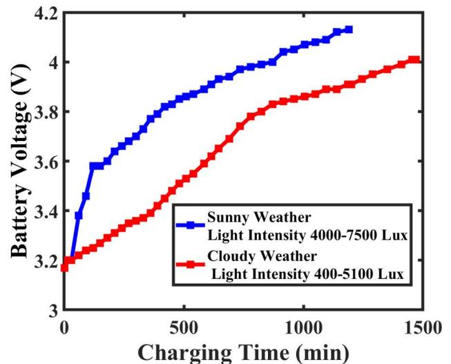
Figure 8: Battery charging using a solar panel on sunny and cloudy days
