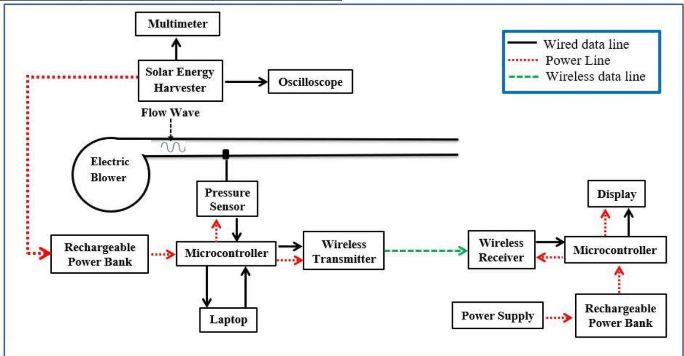
**Figure. 5:** Schematic of experimental setup
