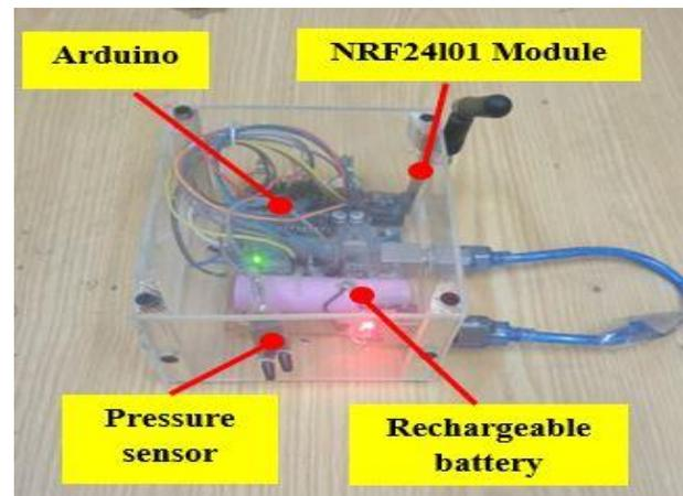
Figure. 3: Wireless transmitter unit
