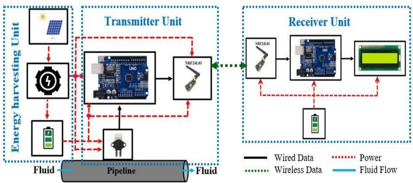
Figure. 2: Architecture of proposed self-powered pipeline monitoring system
