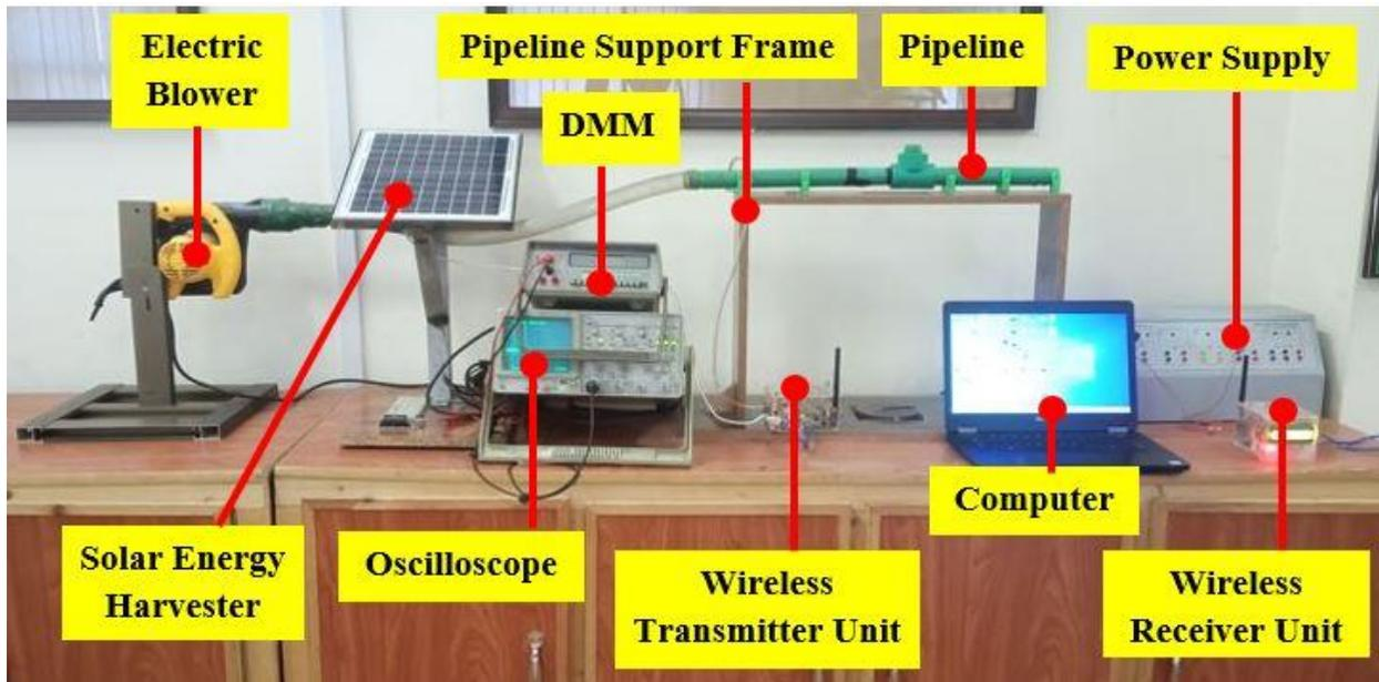
Figure 6: Developed Experimental setup
