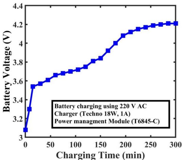
Figure 7: Battery charging using 220 V AC
