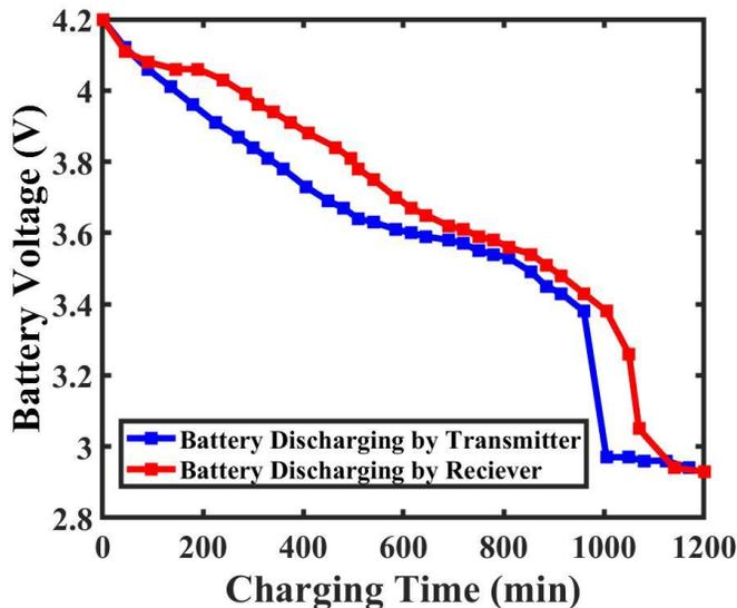
Figure. 9: Battery discharging with transmitter and receiver unit
