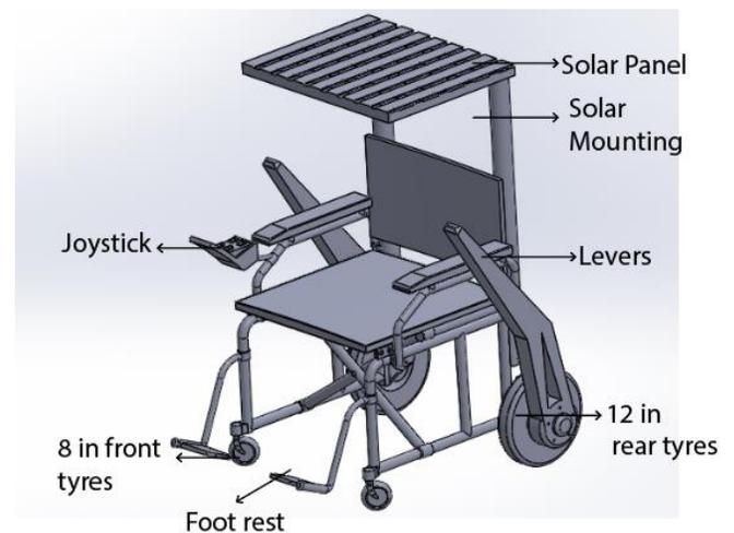
Fig. 2. Conceptual 3D model of HDESW
