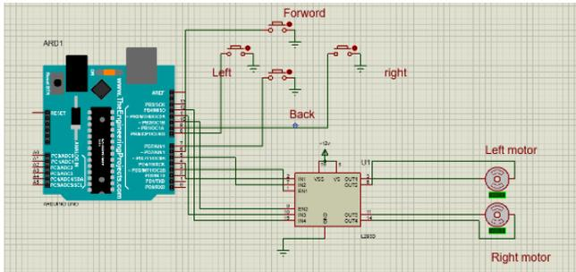
Fig. 5. Electric Drive Schematic in Proteus
