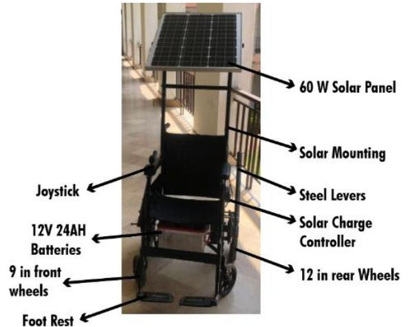
Fig. 4. Photograph of solar/lever drive wheelchair
