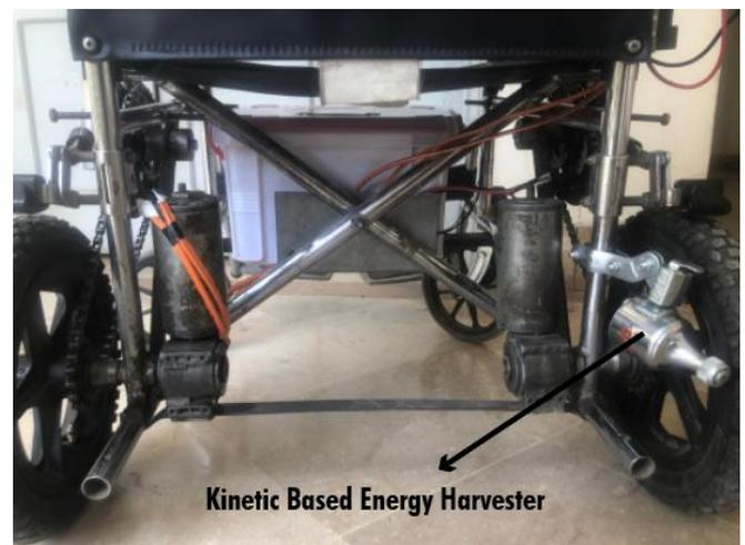
Fig. 7. Photograph of motion based kinetic harvester
