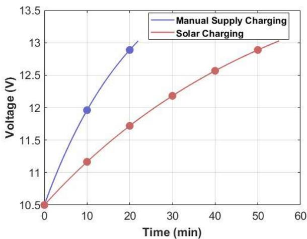
Fig. 8. Charging Behavior of Battery with Time (min)
