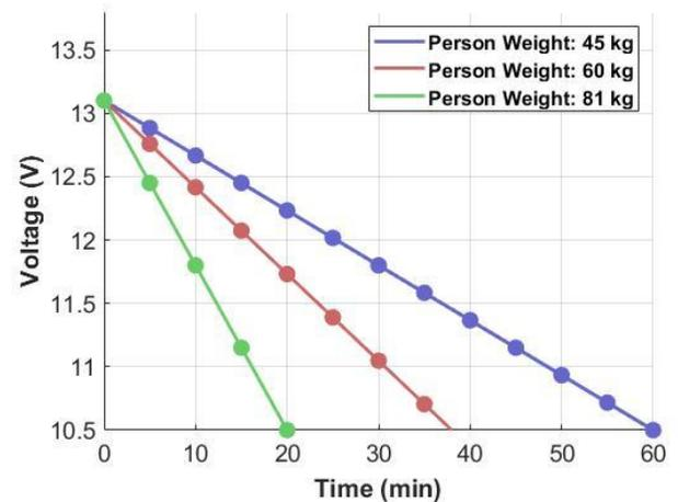
Fig. 10. Discharging Behavior of Battery with Time (min)
