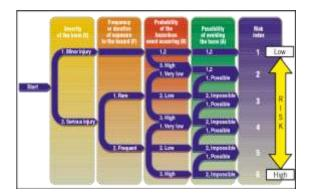
The severity of the harm can be estimated by considering the severity of the injuries or adverse health effects. The proposed choices are:
